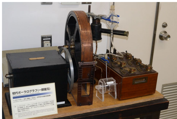
The First Original Polarograph
